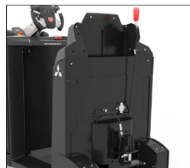
Automatic coupling with ergonomic unlocking handle
