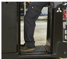
Suspended operator's platform.
